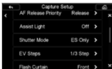
Enabling the Electronic Shutter from the XF Menu.
